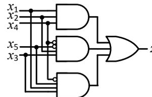
Figure 6. Circuit with weak CI set  $\{x_1, x_2, x_3\}$ .
