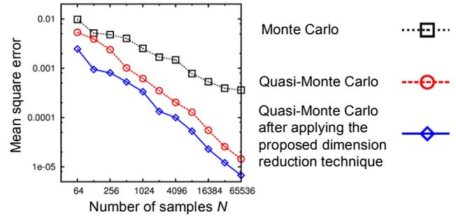
Figure 10. Simulation data for the circuit of Figure 9 showing that dimension reduction significantly decreases MSE.
