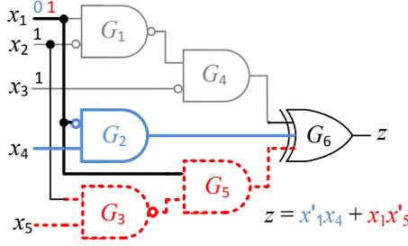
**Figure 4. Five-input circuit; paths from  $x_4$  (blue) and  $x_5$  (red, dashed) are activated by different values of  $x_1$ .**
