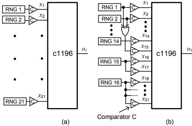
Figure 8. Set-up for SS of the c1196\_o1 benchmark circuit (a) before and (b) after applying dimension reduction.
