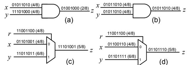
Figure 11. (a) Stochastic multiplier with independent and (b) correlated input bit-streams. Stochastic adder with (c) independent and (d) correlated input bit-streams.
