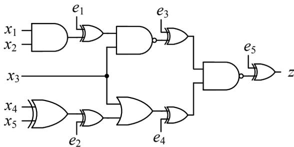
Figure 9. 5-input circuit with XOR gates to model soft errors.
