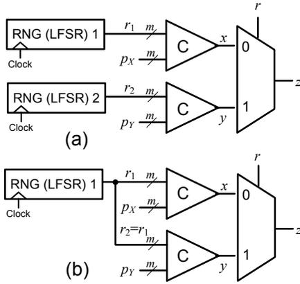
**Figure 12. Dimension reduction in a stochastic adder; (a) with independent RNGs and (b) with shared RNGs.**
