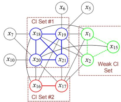
Figure 7. Graph illustrating CI sets of the c1196 benchmark; the clustered nodes can be merged during SS.
