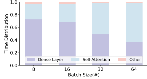
Figure 3. Runtime breakdown of Llama-7b inference with different batch sizes. The dense layer represents the batched K, Q, V generation, O projection, and MLP. The self-attention layer is implemented by FlashInfer (Ye et al., 2024) integrated with PageAttention (Kwon et al., 2023). Results indicate that the dense and self-attention layers together account for over 90% of the execution time, thereby constraining the throughput.
