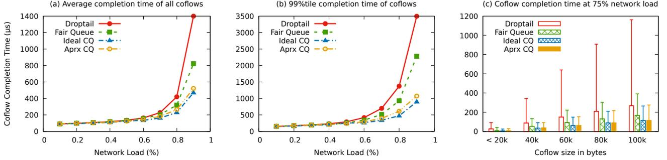
**Figure 8: Coflow completion time when running a mix of background and coflow traffic with coflows prioritized over background flows. (a) average CCT for all coflows, (b) 99<sup>th</sup> percentile CCT for all coflows, and (c) average and 99<sup>th</sup> percentile (using error bar) for various coflow size buckets at 75% network load.**
