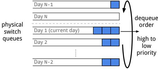
**Figure 1: Example of a Programmable Calendar Queue.**
