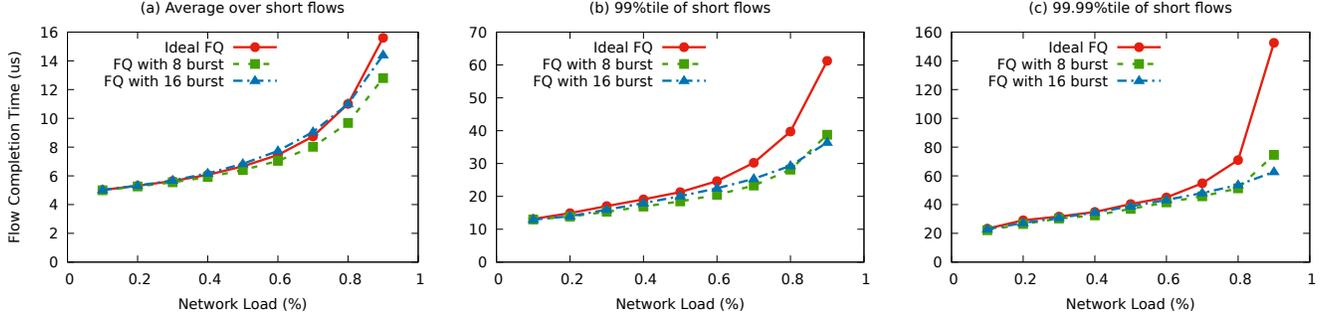
Figure 9: Average and percentile flow completion times for short flows with varying network load and permissible burst size.
