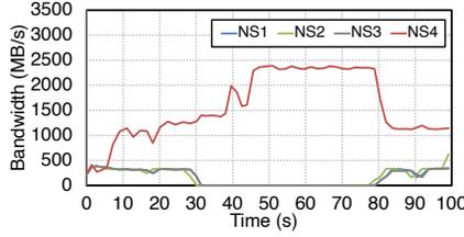
Figure 13: Performance variation of four namespaces with global overdrive under 100s.
