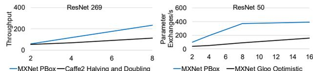
Figure 20: Left: Comparing Caffe2 + Gloo and MXNet + PBox on a 10Gbps InfiniBand network. Right: Comparing MXNet + Gloo and MXNet + PBox on a 56Gbps InfiniBand network with ZeroComputeEngine.
