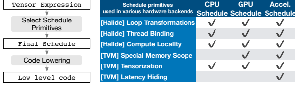
Figure 6: TVM schedule lowering and code generation process. The table lists existing Halide and novel TVM scheduling primitives being used to optimize schedules for CPUs, GPUs and accelerator back-ends. Tensorization is essential for accelerators, but it can also be used for CPUs and GPUs. Special memory-scope enables memory reuse in GPUs and explicit management of on-chip memory in accelerators. Latency hiding is specific to TPU-like accelerators.
