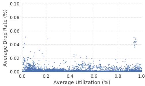
**Figure 1: Scatter plot of ToR-server links' drop rates and utilization across the data center. Drops only include congestion discards and not packet corruptions. Measurements were taken at a granularity of 4 minutes, and samples were taken once per hour over the course of 24 hours.**
