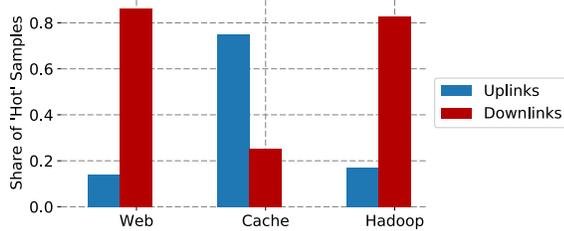
Figure 9: Uplink/downlink share of hot ports given 300 μs sampling.
