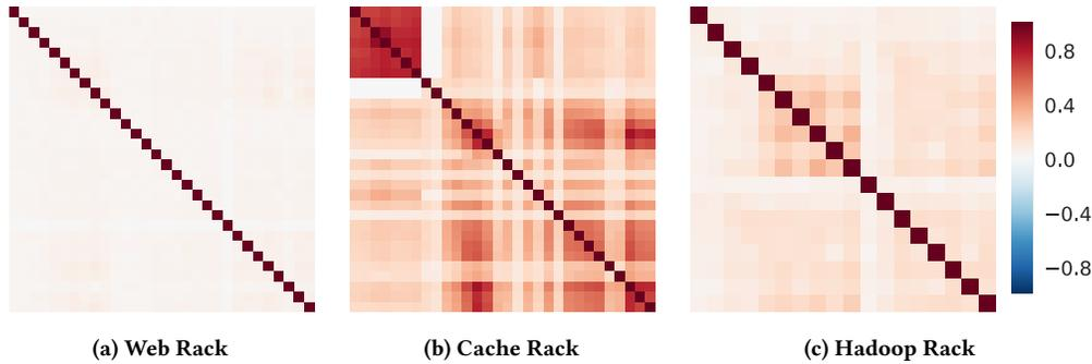
Figure 8: Heatmap of Pearson correlation coefficients for servers in the same rack. We measured the ToR-to-server utilization of three representative racks at a granularity of 250 μs.
