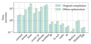
Figure 14: Overhead of DMon-guided optimizations compared to baseline compilation time ( $\sigma < 0.1\mu$ , log-scaled y).
