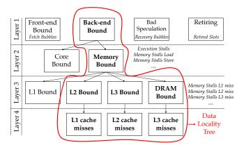
Figure 1: The locality tree abstraction. Performance events that pertain to each tree node are in *italic*. There are no dedicated events to determine if a program is back-end bound. Instead, selective profiling subtracts from total stalls the sum of the stalls that cause other bottlenecks at layer 1 to determine if an execution is back-end bound.
