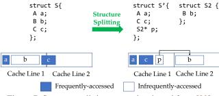
Figure 7: Structure splitting, example adapted from [22].
