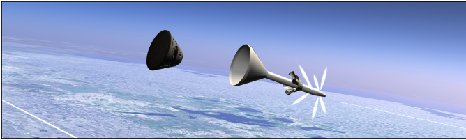
Fig. 8: Orion AA-2 simulation moments after the crew module (left) separates from the launch abort system (right).
