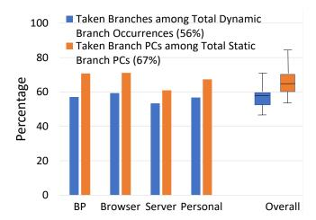
Figure 3: Percentage of static branch PCs and dynamic branch occurrences that are taken.
