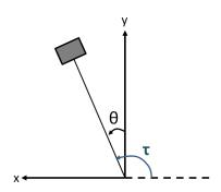
Figure 2.1.1: An inverted pendulum.
