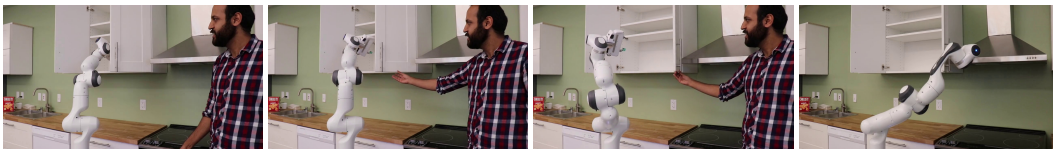
Figure 8: Reactivity. The door handle location is displaced during execution and the robot can be seen to adapting to the new target.
