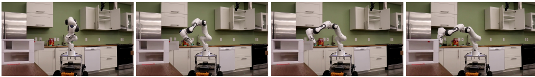
Figure 5: The drawer closing task. The robot successfully closes the drawer from a new initial configuration.
