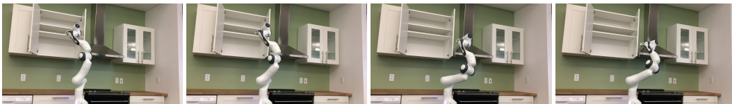
Figure 7: The cabinet door reaching task. The robot manages to reach the cabinet door handle despite of the new initial configuration and new door configuration.
