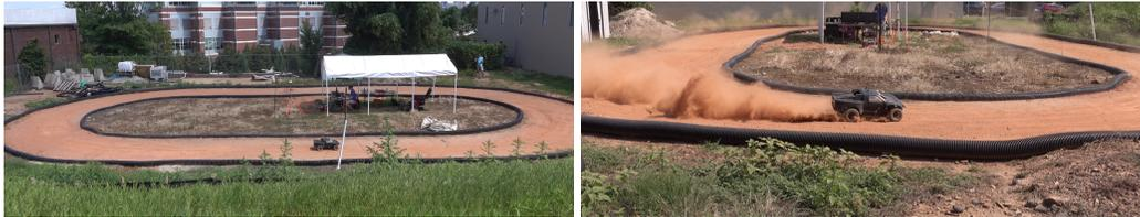
Figure 2: Left: Experimental set-up for AutoRally tests. Right: Drifting around a turn with the MPPI controller and a neural network model.
