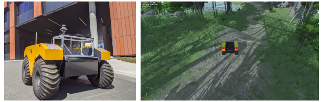
Fig. 7. Left: The University of Washington Clearpath Warthog robot. Right: The 3D skid steering environment that simulates the Warthog. A video of this environment can be found here . The source code for this environment is not publicly available.
