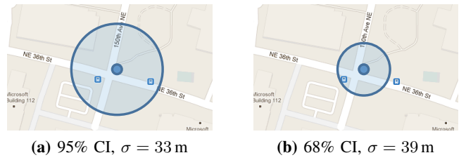
Fig. 1. GPS samples at the same location on two smartphone platforms. Although smaller circles appear more accurate, the sample in (a) is actually more accurate.
