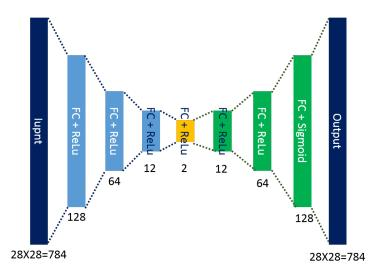
Figure 2: The network architecture of Auto-Encoder.
