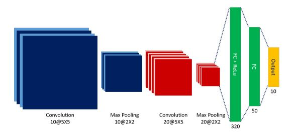
Figure 1: The network architecture of LeNet.
