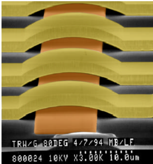
Fig. 3. Top-metal airbridge. To reduce the top-metal trace inductance, we route a small-signal ground strap under the airbridge, as we show in this SEM photo. This ground strap reduces the inductance by 60% to 80%, and doubles the signal propagation velocity, with minimal added capacitance. The typical airbridge trace that we use has a 4\mu\text{m} width, as in this photo.
