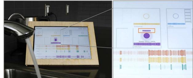
**Figure 2:** A HomeSound IoT display deployed in a home. The red box shows the persistence of sound visualized as a horizontal bar.
