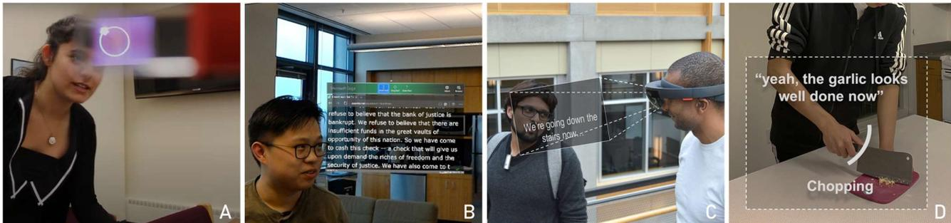
**Figure 3:** Iterative exploration of speech awareness on heads-up displays starting from proof-of-concept localization (A) [6] to an initial captioning prototype (B) [4] to a refined prototype (C) [7] and, finally, a full system combining captions, location, and sound cues (D) [2].
