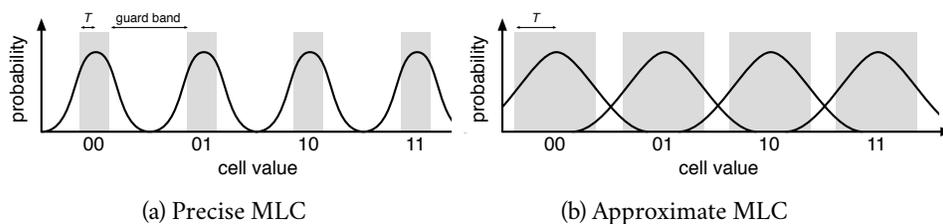
Figure 13: The range of analog values in a precise (a) and approximate (b) four-level cell. The shaded areas are the target regions for writes to each level (the parameter  $T$  is half the width of a target region). Unshaded areas are *guard bands*. The curves show the probability of reading a given analog value after writing one of the levels. Approximate MLCs decrease guard bands so the probability distributions overlap.
