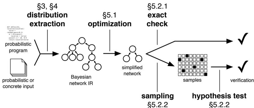
Figure 10: MAYHAP’s workflow to verify probabilistic assertions.
