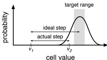
Figure 14: A single step in an iterative program-and-verify write. The value starts at  $v_1$  and takes a step. The curve shows the probability distribution from which the ending value,  $v_2$ , is drawn. Here, since  $v_2$  lies outside the target range, another step must be taken.
