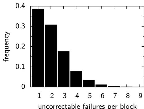
Figure 17: Distribution of uncorrectable cell failures using ECP<sub>2</sub> among 512-bit blocks after the entire memory has been overwritten  $3.2 \times 10^7$  times under the main-memory wear model. (At this stage, half of the blocks have at least one uncorrectable failure.)
