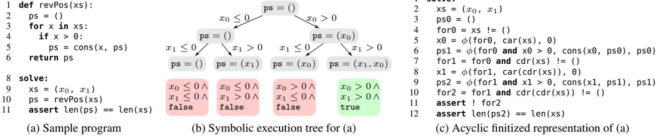
**Figure 5.** Logical encoding of a sample solver-aided query (a), using symbolic execution (b) and bounded model checking (c).
