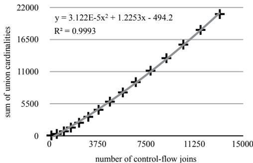
**Figure 10.** SVM performance on B1<sub>v</sub> verification queries, with respect to a range of verification bounds (1 to 15, inclusive). The graph plots the sum of sizes of symbolic unions against the number of control-flow joins encountered during evaluation of each query.
