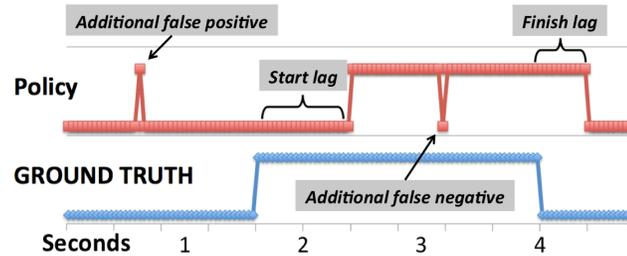
Figure 5.5: **Example Policy Evaluation.** We evaluate start lag (false negatives before a policy is correctly applied), finish lag (false positives after a policy should have been stopped), and additional false positives and negatives outside of these lags.
