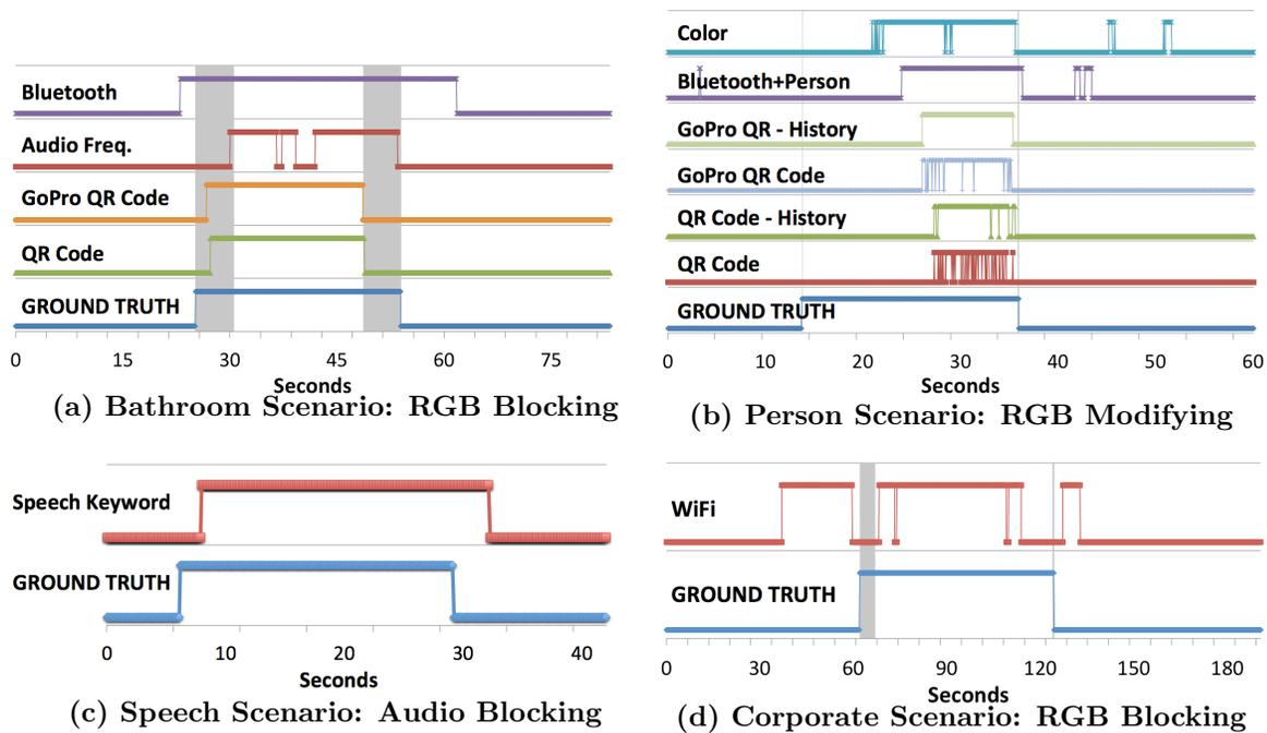
Figure 5.6: **Policy Evaluation.** The grey regions were annotated as “depends” in the ground truth, i.e., the human annotator believed that either blocking or not blocking the event would be acceptable; these events are not counted in Table 5.4. For reference, Figure 5.5 shows an example evaluation.
