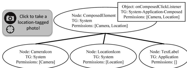
Figure 4.3: **Composition Across Principals.** In this example, the application has composed the system-trusted camera and location icons with its own label to create a custom button that has both camera and location permissions.
