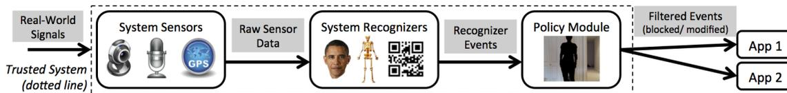
Figure 5.3: **System Overview.** We build on the recognizer abstraction [75], in which applications subscribe to high-level events generated by object recognition algorithms. Our contribution is the policy module (Section 5.4.4), which sees all events, detects policies, and blocks or modifies events accordingly before releasing them to untrusted applications.
