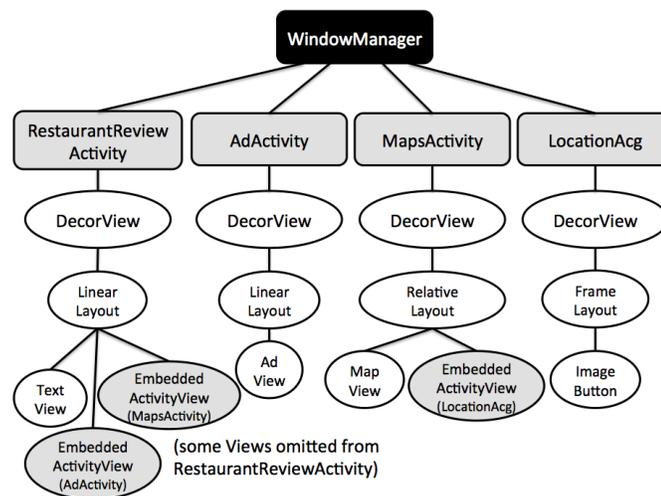
Figure 4.5: **Window Management.** This figure shows the Window/View tree for the Activities in Figure 4.4. Embedded Activities are not embedded in the View tree (circles) of their parent, but rather within a separate window. The WindowManager keeps track of a window (grey squares) for each Activity and visually overlays an embedded window on top of the corresponding EmbeddedActivityView in the parent Activity.
