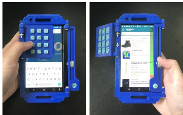
Figure 1. Interactiles allows people with visual impairments to interact with mobile touchscreen phones using physical attachments, including a number pad (left) and a multi-purpose physical scrollbar (right).
