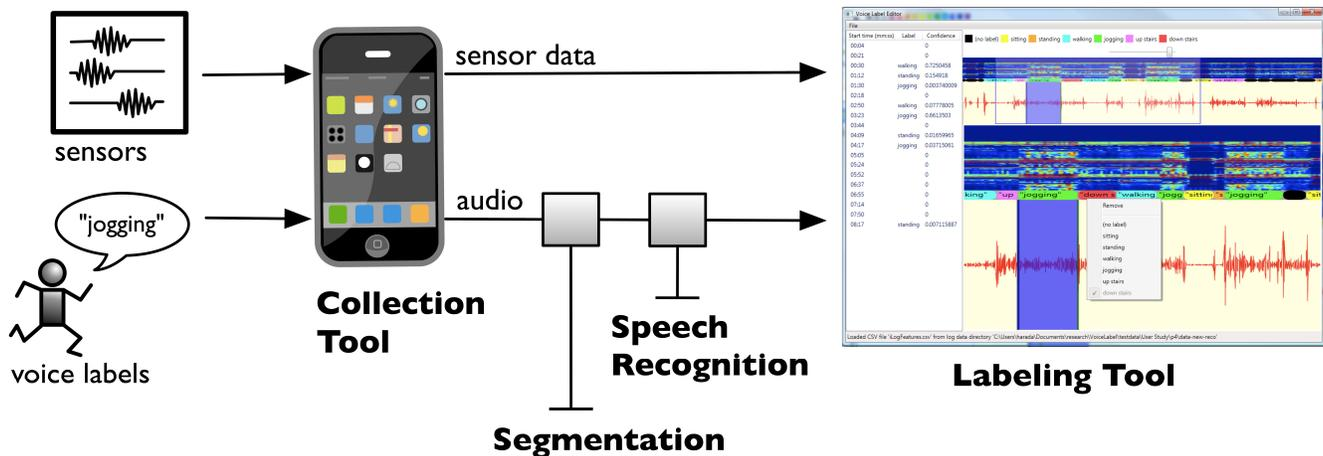
**Figure 1: The VoiceLabel architecture. A mobile collection tool gathers sensor data and voice labels as the data collector engages in various activities. The collected data is processed through a segmentation module that identifies the activity transition points and a speech recognition module which attempts to extract the uttered label. The result can be viewed and manipulated via the labeling tool.**
