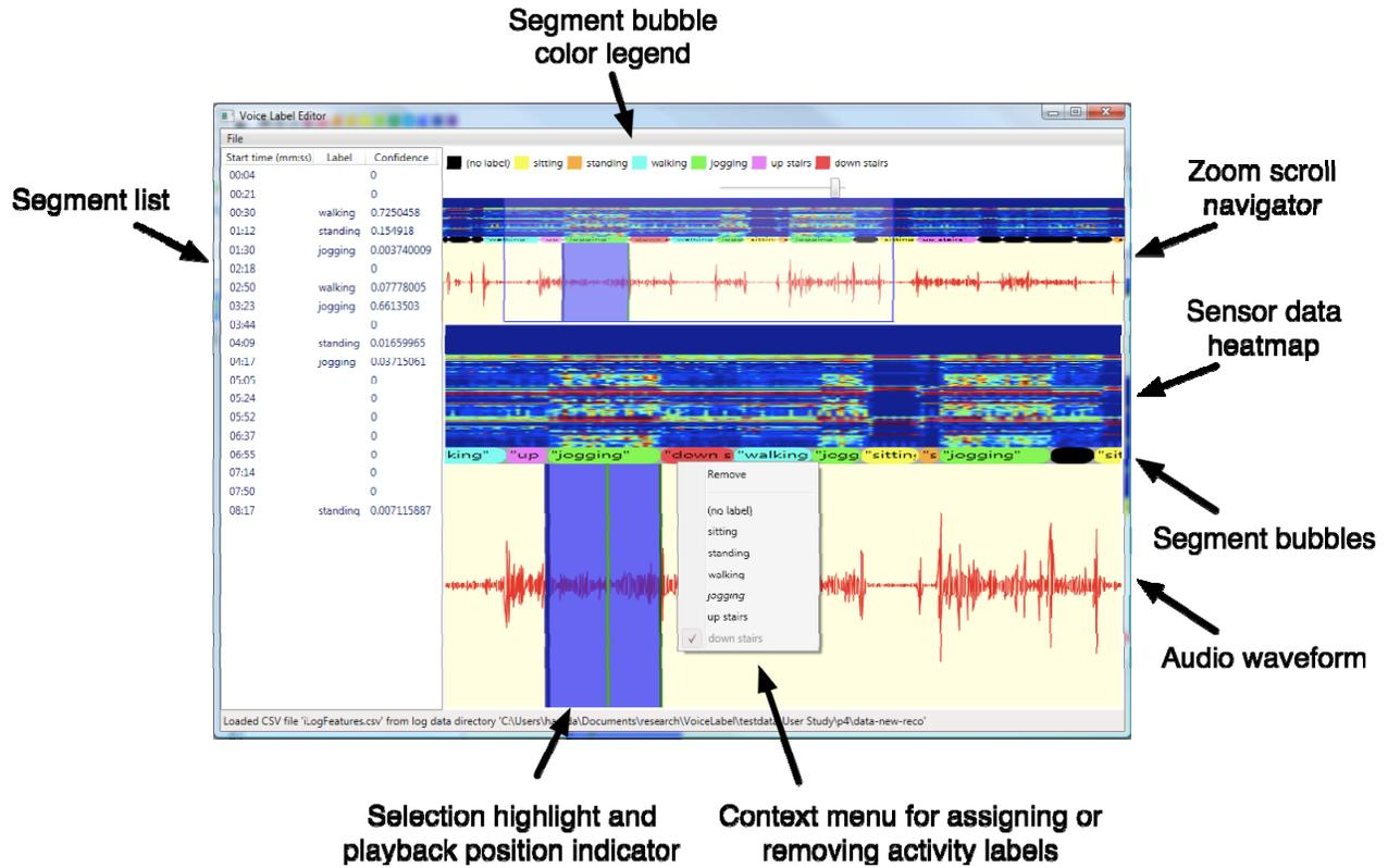
**Figure 2: Screenshot of the VoiceLabel labeling tool. The tool allows the labeler to easily browse through the sensor data recorded during the data collection phase, along with the audio waveform containing the activity labels. It also automatically extracts activity transition points as segment bubbles containing the recognized activity label; these automatic labels can be corrected if, after listening to the corresponding audio, they are determined to be incorrect.**
