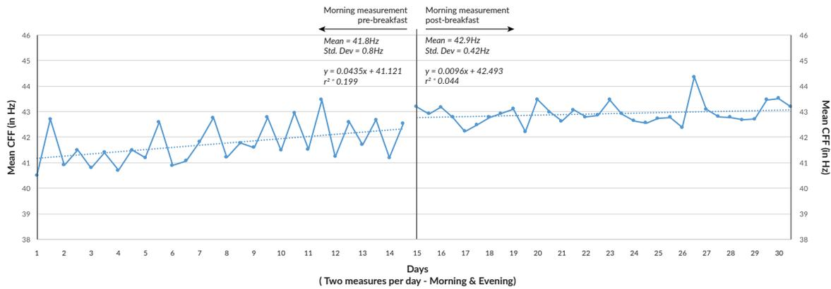
Fig. 11. Month-long CFF measurement data collected by member of the research team using *Beacon*. Measures were taken twice daily—morning and evening. After 2 weeks, the morning measurement time was pushed back to see if the change in wakefulness would be picked up by *Beacon*. *Beacon* successfully picked up the slight variation in wakefulness, providing evidence of potential for long term CFF tracking.
