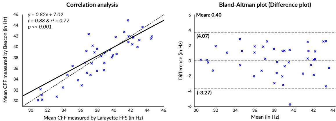
Fig. 10. Analysis of comparative study evaluating the performance of *Beacon* when compared to the Lafayette FFS. Left: Regression analysis shows a strong correlation between the CFF measure by *Beacon* and Lafayette FFS with a Pearson’s R of 0.88. Right: The Bland-Altman plot shows the mean difference between *Beacon* and Lafayette FFS to be 0.4Hz with a maximum difference of at most  $\pm 3.67$ Hz for 95% of the measurements.
