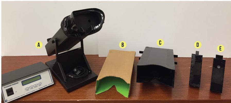
Fig. 5. Stages of the iterative design process for *Beacon*. Left: (A) Lafayette FFS, the golden standard device that informed our design of *Beacon*. Right: (B) Cardboard prototype, (C) Acrylic prototype with adjustable distance between light source and eyes, (D) portable prototype, and (E) portable prototype with guiding lights for horizontal and vertical alignment.
