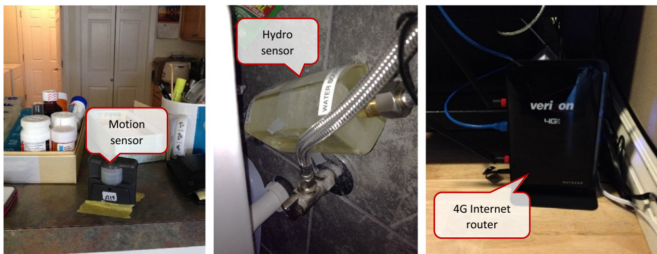
FIGURE 1 A deployment of a home-based sensor system in one of our study sites. (Left) motion sensor in a dining room; (Middle) hydro sensor in a bathroom; (Right) Internet router in a living room. Please note that these are actual pictures, not staged pictures
