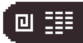
Figure 4. Our current marker locator pattern and identifier pattern. Bits three and fifteen are active.
