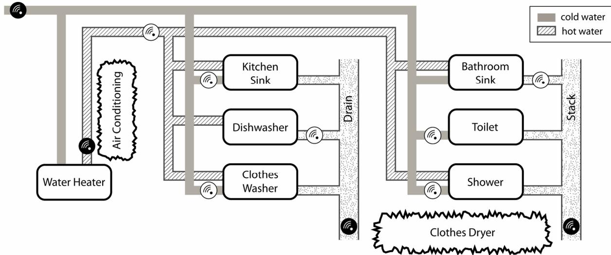
**Figure 1. Schematic of the water pipes in the home where we conducted our feasibility study. The air conditioning and clothes dryer are shown because they rattled nearby pipes, introducing noise that needs to be considered in analyses. The four shaded sensors are used for modeling activities, while the unshaded sensors are included only for validating our results.**
