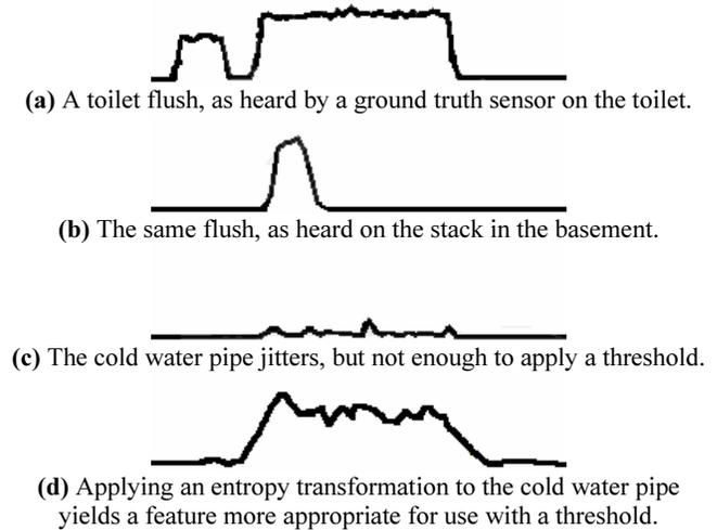
**Figure 3.** Several signals obtained from our sensors.
