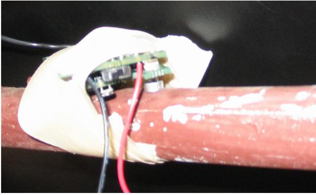
**Figure 2.** Our prototype sensor attached to a water pipe. The microphone is the cylinder in the center. We pressed the microphone against the pipe and secured the sensor with tape.
