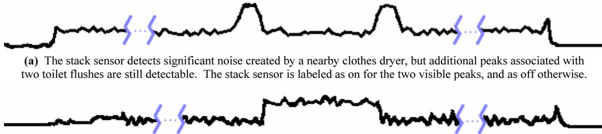
(a) The stack sensor detects significant noise created by a nearby clothes dryer, but additional peaks associated with two toilet flushes are still detectable. The stack sensor is labeled as on for the two visible peaks, and as off otherwise.
