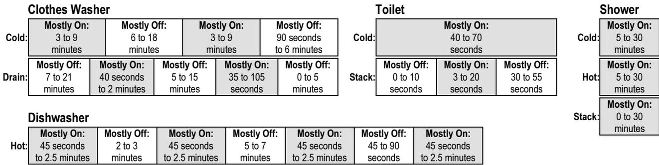
Figure 6. Clothes washer, dishwasher, and toilet activity are matched based on the mechanical patterns in their water usage. Showers are the only activity that continuously use hot and cold water while generating waste water for an extended period of time.
