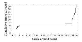
**Figure 10.** To test error correction, we moved a droplet in circles until failure. Total experiment time was 2 hours and 11 minutes. Along the way, the computer vision system detected and corrected errors, marking regions of the board as faulty and avoiding them in the future. The errors at the beginning correspond to faulty electrodes; those at the end were caused as the droplet evaporated.
