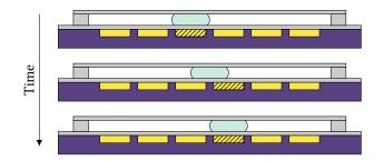
**Figure 3.** Side view of the PurpleDrop DMF device. Electrodes (yellow) sit at the top of the PCB (purple) in a grid. The PCB is topped with a dielectric and hydrophobic layer. The top plate sits on risers and is also hydrophobic and conductive. Droplets are attracted to the activated electrodes (shown with diagonal lines). Activating the neighboring electrode will move a droplet.
