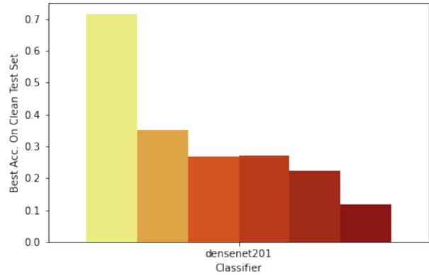
Figure 11. Best achievable accuracy after 50 epochs across a range of hyperparameters and random seeds for the pixel-based approach after applying aggressive training-time augmentations.  $\mu = 0$  corresponds to the unmodified, clean dataset for this approach.
