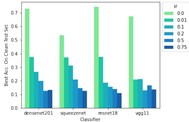
Figure 6. Best achievable accuracy after 50 epochs across a range of hyperparameters and random seeds for the pixel-based modification.  $\mu = 0$  corresponds to the unmodified, clean dataset for this approach.
