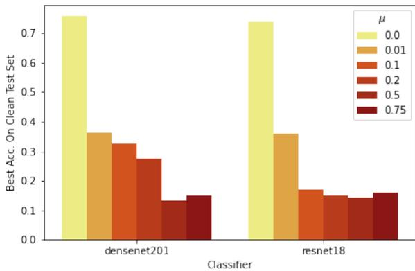
Figure 10. Best achievable accuracy after 50 epochs across a range of hyperparameters and random seeds for the pixel-based approach after applying Gaussian noise to the images.  $\mu = 0$  corresponds to the unmodified, clean dataset for this approach.
