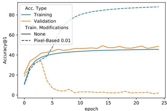
Figure 1. ResNet18 train and validation accuracy on ImageNet protected with the pixel-based modification at  $\mu = 0.01$ , compared with unmodified ImageNet. Validation accuracy can reach up to 70% with unmodified data, but our modified dataset prevents effective learning within the first several epochs.
