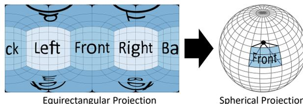
**Figure 1: An equirectangular frame encoded within each 360° video (left) and its projection onto a sphere. Only a small portion of the sphere is within a user's field of view at any time.**
