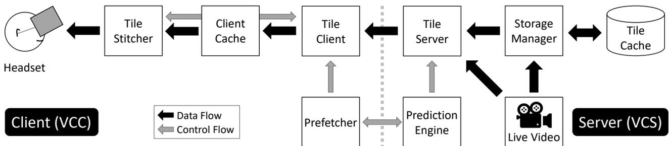
**Figure 3: The VisualCloud architecture.** The server-based components (VCS) are responsible for ingesting, segmenting, transmitting, and storing video. The VCC requests tiles in prediction-based order, stitches segments together, and displays the result on the headset.
