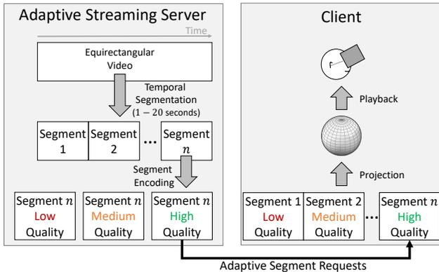
**Figure 2: Adaptive streaming in a VR context. On the server, a video is temporally segmented into 1-20 second slices. Each slice is encoded at various qualities. A client then requests segments at a given quality based on network congestion. Segments are concatenated, projected, and rendered on a headset.**
