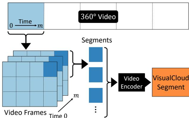
**Figure 4: The video spatiotemporal segmentation process, used both in the storage manager and during in-memory stream processing.** 360° videos are segmented in time and then spatially decomposed into segments. Each segment is stored as a single encoded fragment.
