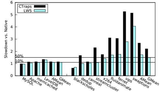
Figure 9: Runtime overhead of CTraps and LWS.
