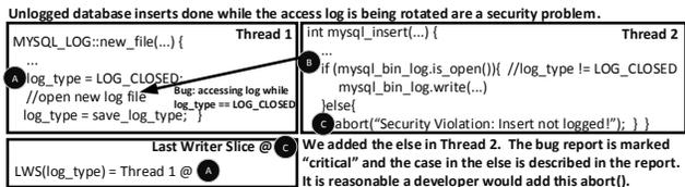
**Figure 8:** Using last writer slices to debug an atomicity violation in MySQL 4.0.12. The last writer slice reveals the code that closes the log before a database insertion that goes unlogged, which is a security problem.
