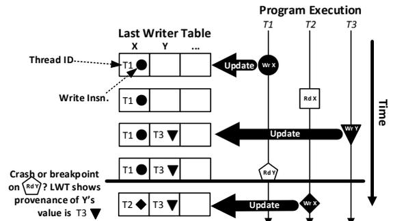
**Figure 3:** Basic operation of the last writer table. Different shapes signify different distinct memory operations.
