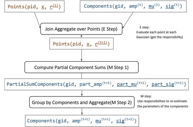
**Figure 4: Query plan showing the optimized implementation of an EM algorithm for GMM in Myria. The relations are represented by sharp cornered boxes, and the operators by rounded boxes. This query plan performs one EM step, updating the parameters of the Gaussian components from time  $(t)$  to  $(t + 1)$ .**
