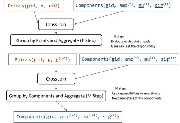
**Figure 3: Query plan showing the naïve implementation of an EM algorithm for GMM in Myria. The relations are represented by sharp cornered boxes, and the operators by rounded boxes. This query plan performs one EM step, updating the parameters of the Gaussian components from time ( $t$ ) to ( $t + 1$ ).**
