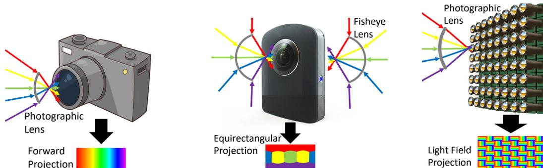
(a) **Photographic camera.** A two-dimensional photographic camera with a field of view defined by its lens and other physical characteristics. A forward projection is used to map light rays onto a plane.
