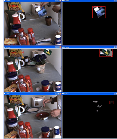
Figure 4. Examples of segmentation results, with the left and right row being original frame and segmented result, respectively. Only pixels in the biggest connected component (depicted by the rectangle) are used. The three rows are examples of good, moderate, and bad segmentation results, respectively.
