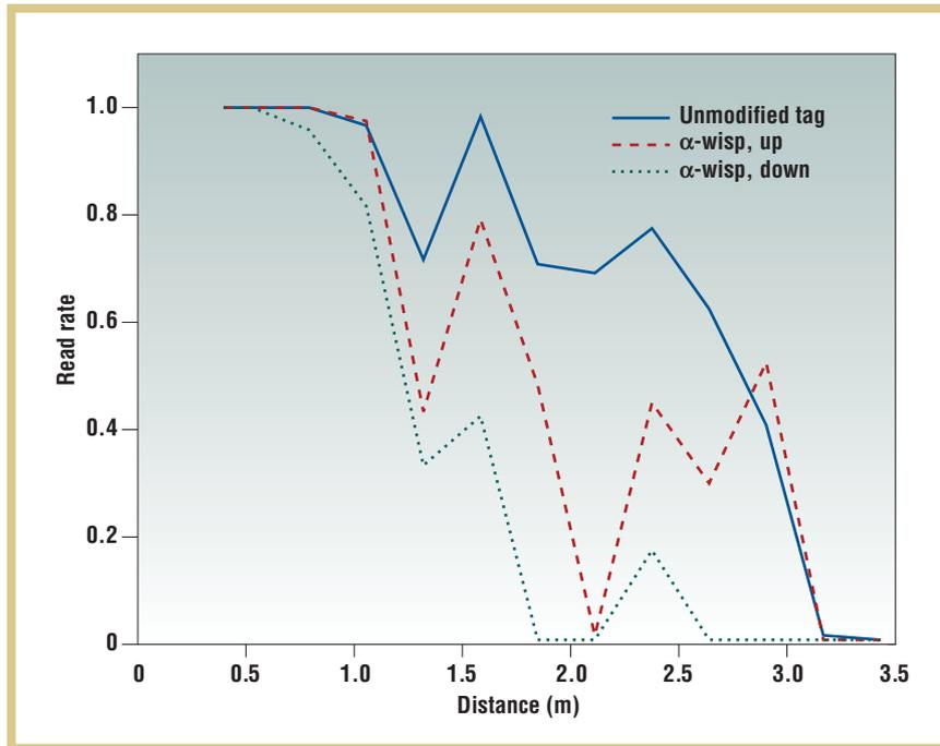
**Figure 2.** The dependence of read rate on read distance. Data is for an  $\alpha$ -wisp serial-switch configuration. Read rate is the fraction of reads in which the reader detected a single stationary tag with no occlusion in typical indoor conditions.  $\alpha$ -wisps are detectable beyond 3.0 meters from the reader. Read rates are lower than for unmodified RFID tags.
