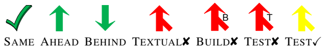
Figure 3: Crystal associates an icon with each of the seven relationships. The color of each relationship icon represents the severity of the relationship: relationships that require no merging are green, that can be merged automatically are yellow, and that require manual merging are red.
