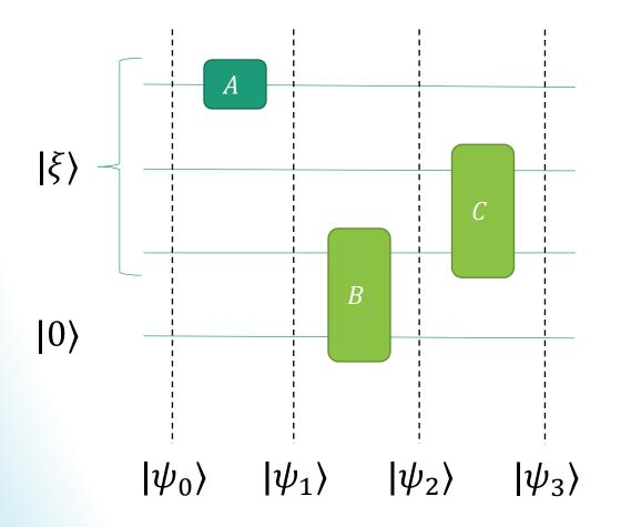
$\begin{aligned} |\psi_0\rangle &= |\xi\rangle |0\rangle \\ |\psi_1\rangle &= A |\psi_0\rangle \\ |\psi_2\rangle &= B |\psi_1\rangle \\ |\psi_3\rangle &= C |\psi_2\rangle \end{aligned}$
