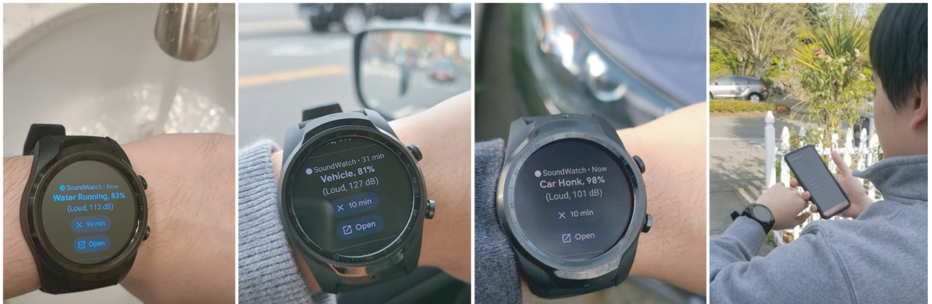
Figure 1. Different use cases of our SoundWatch sound classification app and one of the four architectures (watch+phone).
