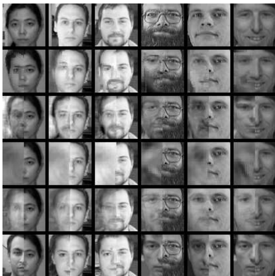
Figure 5: Sample face completions. Top to bottom: original, SPN, DBM, DBN, PCA, nearest neighbor. The first three images are from Caltech-101, the rest from Olivetti.
