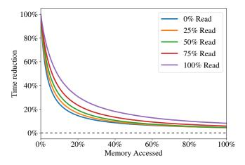
Figure 8. Total cost to create process and access a portion of the allocated memory. The different lines represent different mixtures of read and write accesses. For example, "25% Read" implies 75% write. The values are the average of 10 experiment runs.
