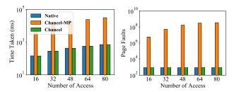
**Fig. 11:** (a) Average completion time and (b) the total number of EPC page faults when the number of memory accesses to each EPC page increases linearly. CHANCEL is  $37.88-48.08\times$  faster than CHANCEL-MP and incurs an overhead of only 0.1-0.8% compared to NATIVE.
