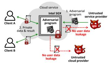
**Fig. 1:** CHANCEL's system model with three participants: the clients, the service provider, and the cloud provider. CHANCEL must prevent the service provider's adversarial program that uses multi-threading to concurrently serve many clients, from leaking confidential client data.
