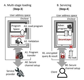
Fig. 2: Overall workflow of CHANCEL. A) An enclave containing SecureLayer is created, which then validates and loads a program provided by the service provider. B) The runtime behavior of the program is restricted, and SecureLayer mediates all interactions originating from it to avoid any security threat.
