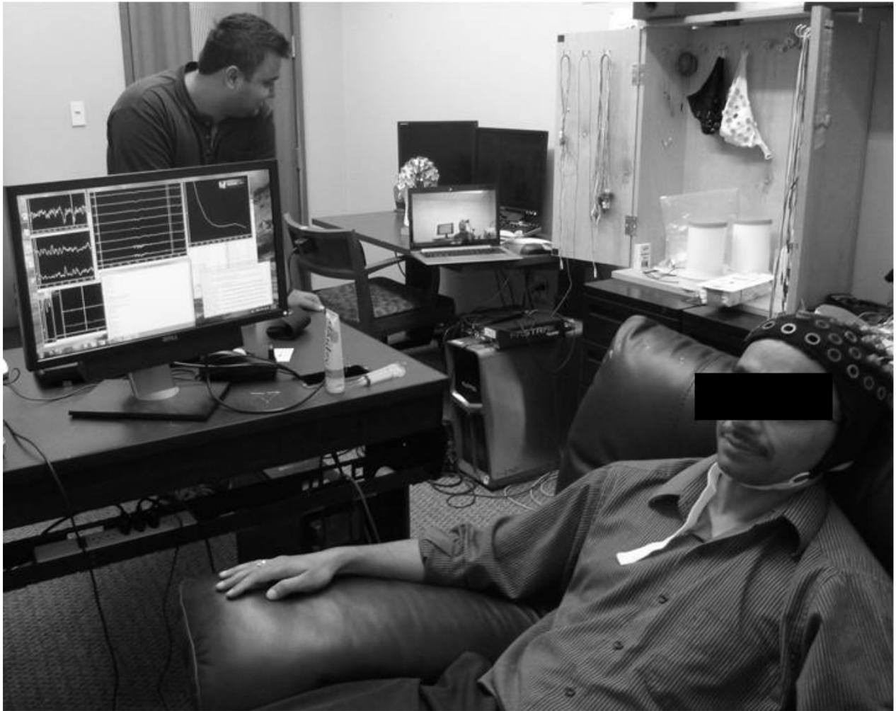
**Figure 2. EEG Set-Up.** EEG signals being recorded from a subject (the "Sender") as the subject watches the computer game (the game screen is to the left and not shown in the picture). The larger screen displays EEG signals processed by the BCI2000 software. The smaller laptop screen placed further away is from the live Skype session and shows a "Receiver" subject in the TMS lab across the University of Washington campus. (Image from the pilot study referred to in the text).
