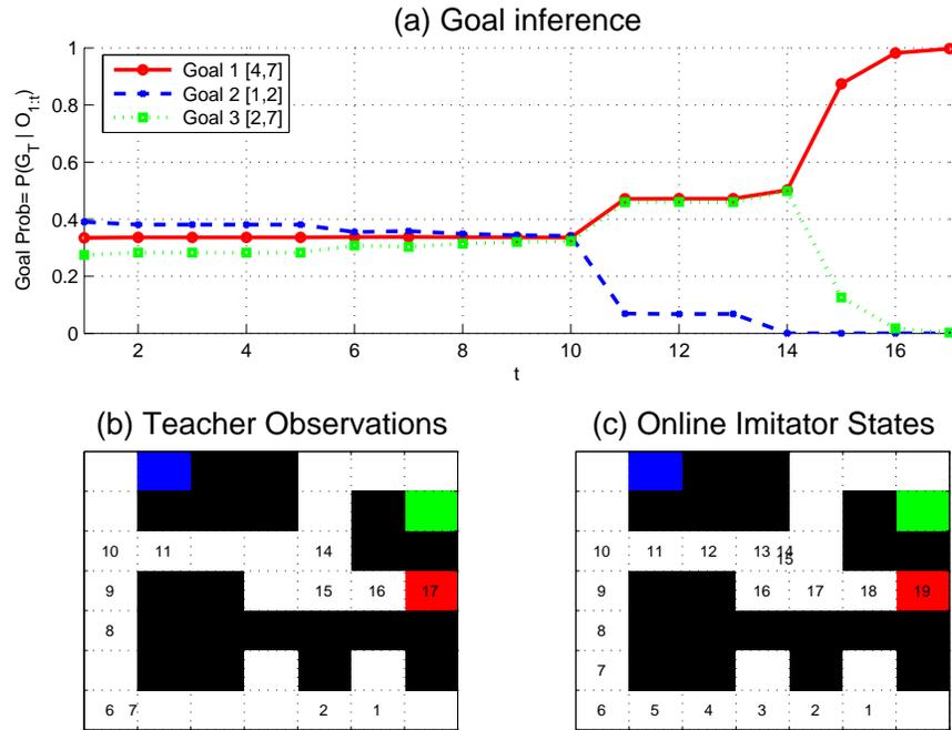
Figure 6: **Online Imitation with Uncertain Goals:** (a) shows the goal probabilities inferred by the agent at each time step for the noisy teacher trajectory in (b). (b) Observations of the teacher. Missing numbers indicate times at which the teacher was occluded. (c) The agent is able to follow the teacher trajectory even when the teacher is occluded based on the evolving goal distribution in (a).
