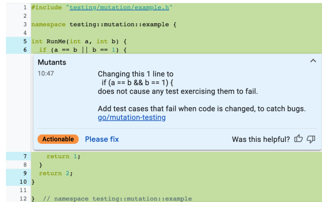
Figure 1: A mutant surfaced in the code review tool. A reviewer can click “Please fix”, indicating that the author should resolve the mutant. Both author and reviewers can click “Thumbs up” and “Thumbs down” to give feedback.
