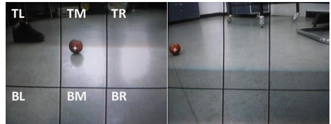
Figure 1: Robot's point of view. Left - go forward area; Right - turn left and go forward area.
