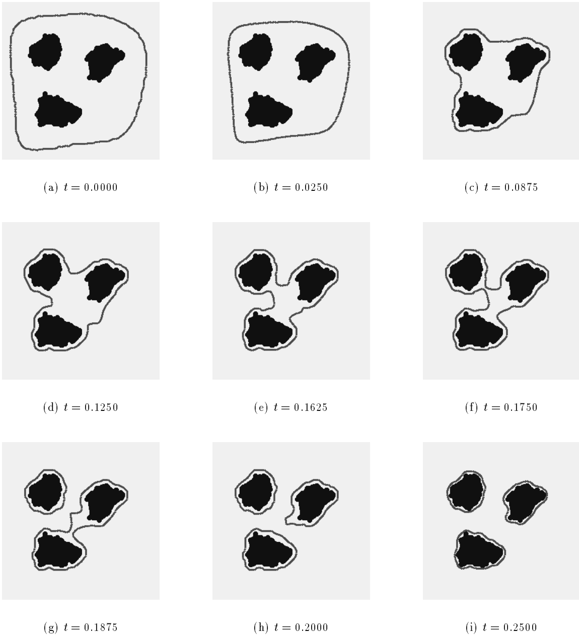
Figure 12: Topological split: a single instance of the shape model splits into three instances to reconstruct the individual shapes. Computation was done on a 64 \times 64 mesh with a time step \Delta t = 0.00025 .
