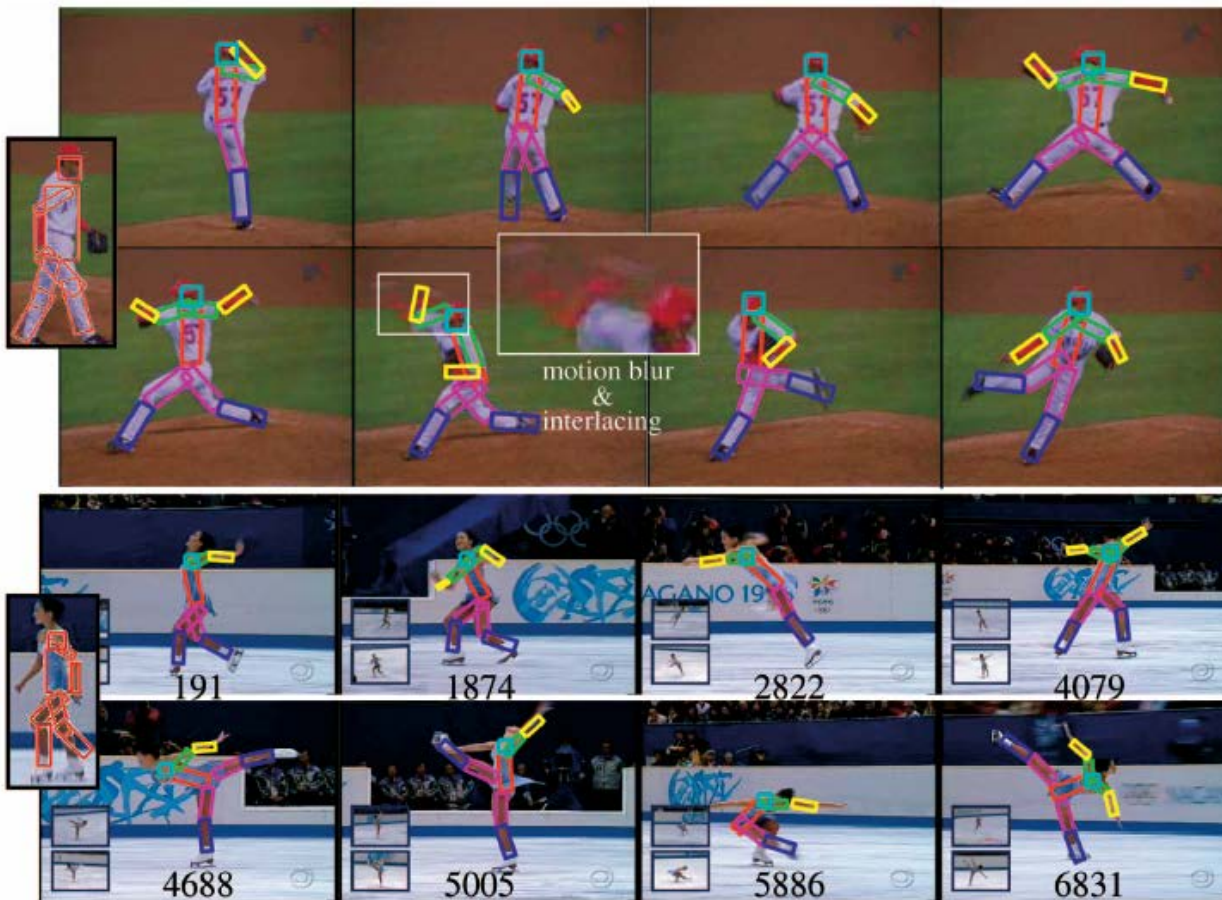
Fig. 22. Our automatic tracker on commercial sports footage with fast and extreme motions. On the top , we show results from a 300 frame sequence of a baseball pitch from the 2002 World Series. On the bottom , we show results from the complete medal-winning performance of Michelle Kwan from the 1998 Winter Olympics. We label frame numbers from the 7,600-frame sequence. For each sequence, our system first runs a walking pose finder on each frame; and then uses the single frame with the best score (shown in the left insets) to train the discriminative appearance models. In the baseball sequence, our system is able to track through frames with excessive motion blur and interlacing effects (the center inset). In the skating sequence, our system is able to track through extreme poses for thousands of frames. This means that our system can track long sequences with extreme poses, complex backgrounds, and fast movement without manual intervention .
