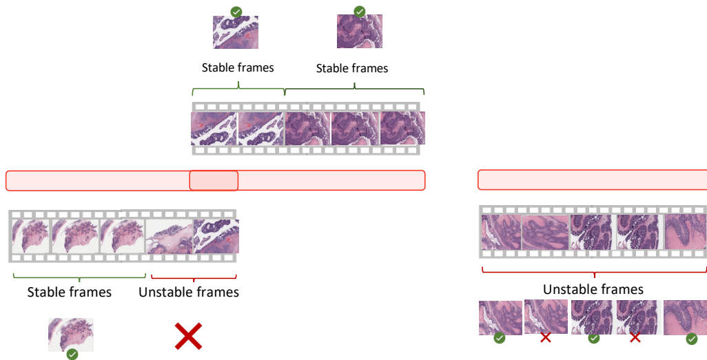
Figure 13: Representative Frame Identification. If a Stable frame is found by Algorithm 1 within the candidate regions, we use it as the representative frame. If not, we use the most dissimilar frames among unstable frames.
