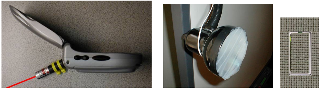
Figure 4: On the left, a laser instrumentation of Motorola iDEN i95cl. In the middle, an example of a long-range active tag that responds and decodes. On the right, a prototype of an active tag embedded within a light switch and wall plate.
