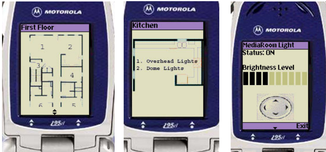
Figure 3: Screenshots of Universal Remote at different modes of control (floor level, room level, and device level)
