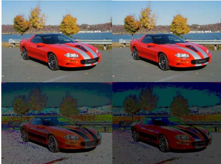
**Figure 4:** An example of metadata encoded in each 8 bit RGB value for each pixel. Top left: Original Picture. Top right: Metadata encoded in 1 LSB. Bottom left: Metadata encoded in 2 LSBs. Bottom right: Metadata encoded in 3 LSBs.
